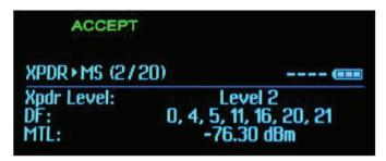
The 20-character 4-line display provides for easily viewable data and parametric measurements as required for Mode S Elementary and Enhanced Surveillance testing. For legacy test modes, the menu structure and displayed data format have been retained so that minimal changes are required of fielded procedures.
